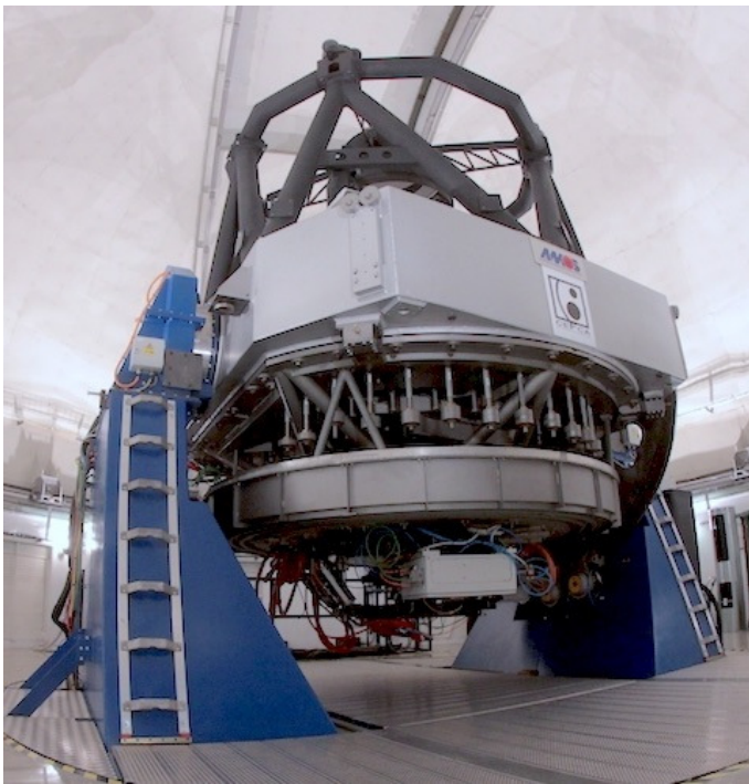
Fig. 1: View of the JST/T250 telescope, the primary telescope of the OAJ. It is the telescope used for the miniJPAS survey, with the JPAS-Pathfinder camera integrated at the Cassegrain focus.
