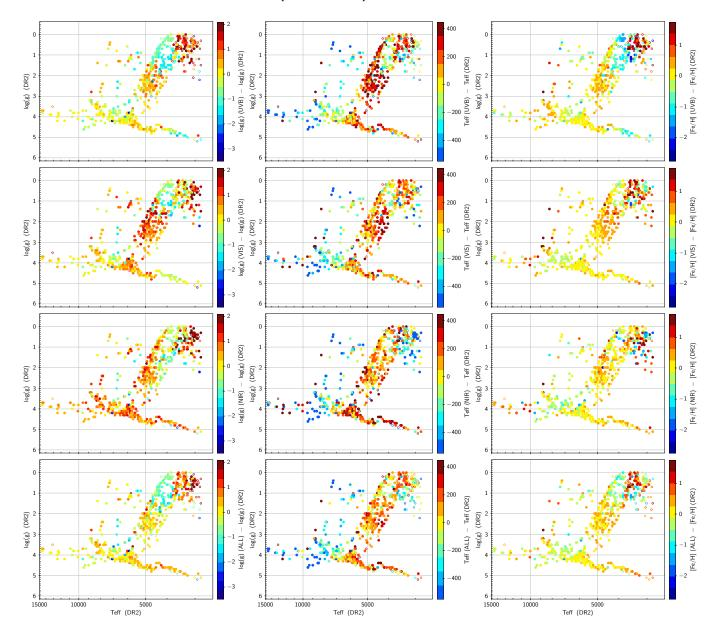
**Fig. 9.** Trends in the differences between the parameters of DR2 and those from best-matching GSL SEDs as a function of position in the HR diagram. The data in the *left column* are colored by difference in  $\log(g)$ , the *middle column* by difference in  $T_{\text{eff}}$ , and the *right column* by difference in [Fe/H]. From top to bottom, the spectral ranges used for the comparison with GSL are the UVB, the VIS, the NIR, and all three arms of X-shooter.
