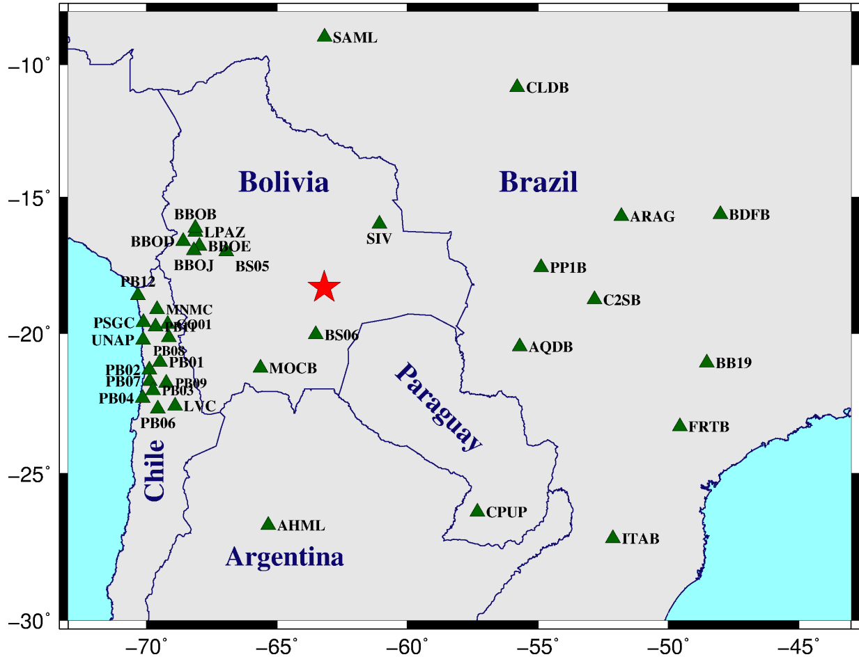
Figure 2.3: Santa Cruz de la Sierra earthquake (red star) and stations (green triangle) up to a distance of 15^\circ utilized to do the relocation with the iLoc program. Arrival times were taken from ISC catalog ( International Seismological Centre, 2013b ).
