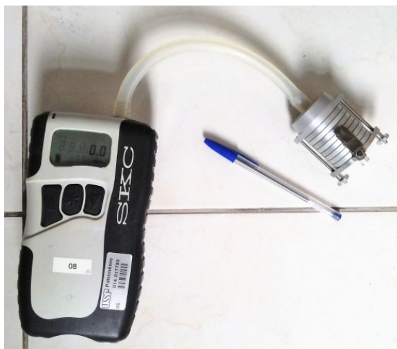
Figure 4. Photograph of the Personal Cascade Impactor Sampler (PCIS) and the Leland Legacy Sample Pump (SKC).
