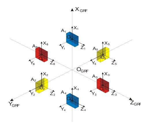
Figure A.1: Notation and location of the 6 accelerometers of the GOCE gradiometer in the GRF and with all 6 ARF's. The axes of the ARF shown by solid arrows are aligned with ultra sensitive axes of the accelerometer. The axes of the ARF shown by dashed arrows are aligned to the less sensitive axes of the accelerometer. Each colour represents a one-axis gradiometer. The shadowed surfaces represent the locations of the lower plates (and the sole plates).
