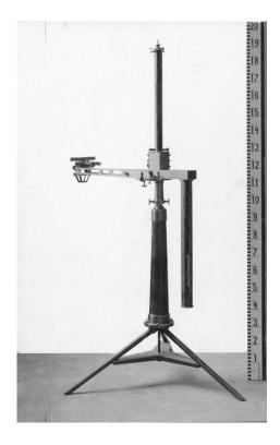
Figure IV-1: Single Eötvös' Torsion Balance designed for field work. The first Gravity Gradiometer. Courtesy of the Loránd Eötvös Geophysical Institute (Szabo, 1998).
