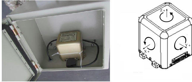
Figure 3.3: Photograph of the IMU Motion Pack III and a schematic diagram of the coordinate axes.
