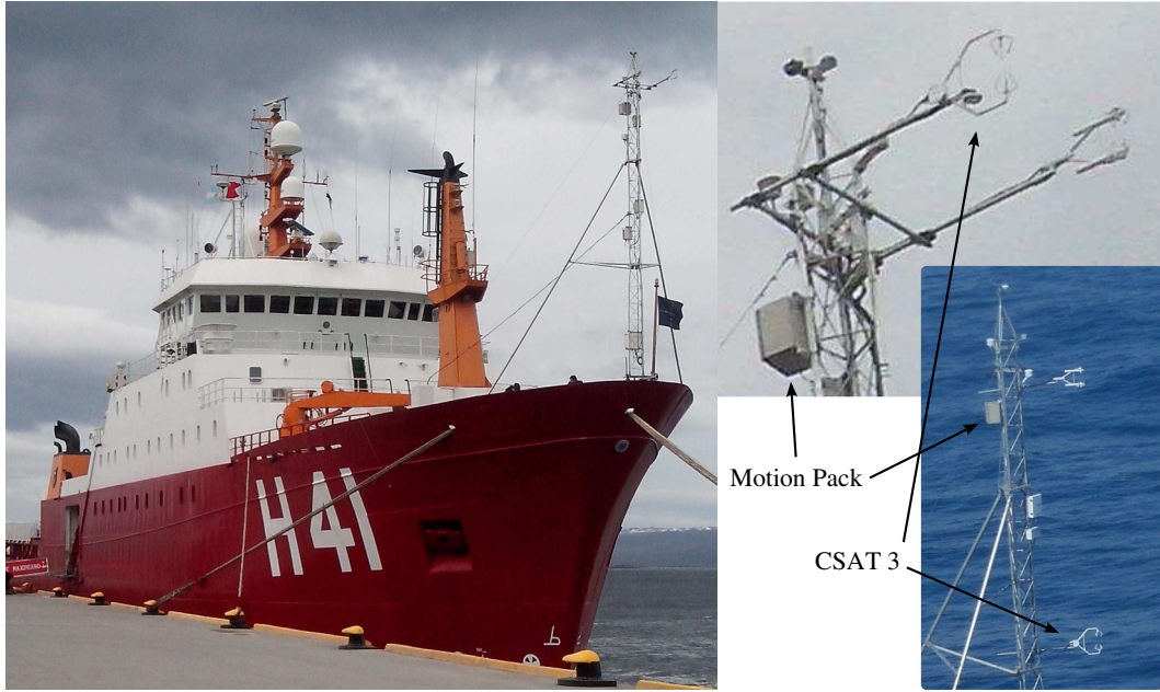
Figure 3.2: Photograph of the Polar Ship Almirante Maximiano H-41 taken in October 2014 (left) and instrumentation set-up for both the OP32 and OP33 campaigns (upper right), and for the OP34 campaign (lower right), showing the two sensors used in this work: the IMU Motion Pack III and the sonic anemometer CSAT 3.
