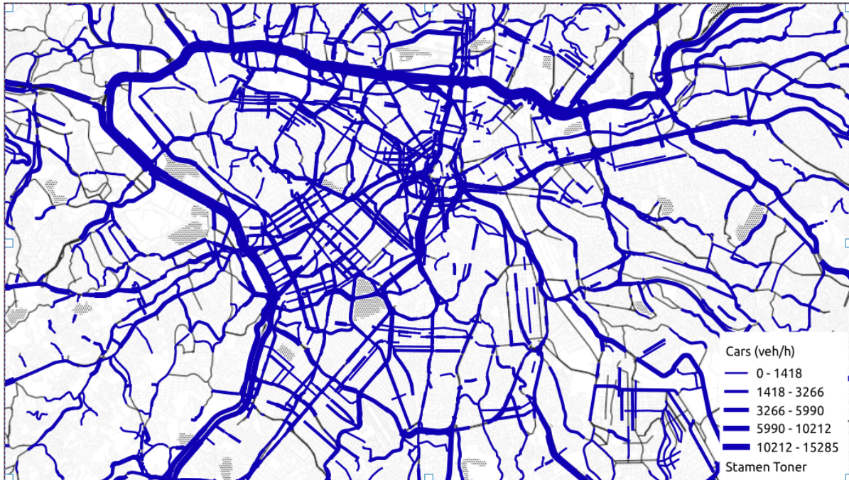
Figure 32 – Traffic flow of Cars generated from GPS data with spatial correction using speed as proxy ( veh \cdot h^{-1} ).
